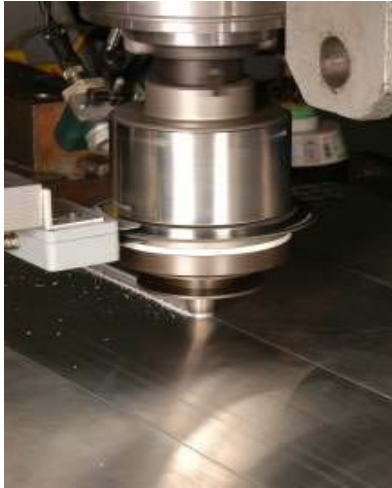
Original system in action incorporating revolving antenna and static receiver
